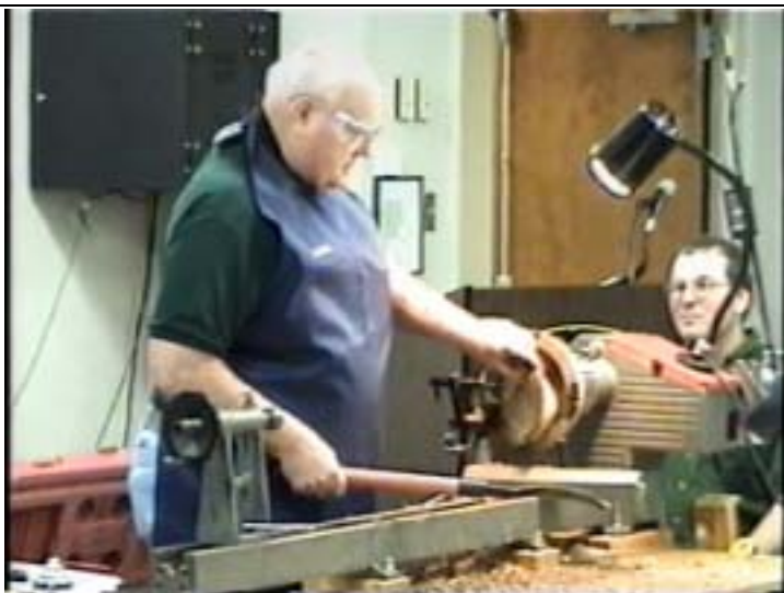
A little pressure and the first coring is removed....
