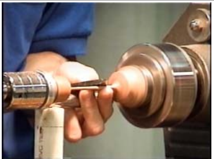
He used a very large skew to turn the thin stem
