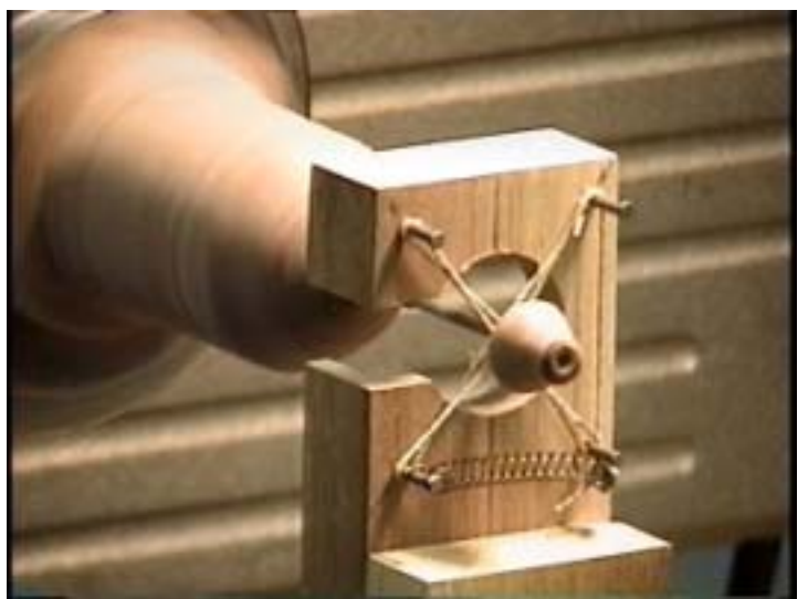
A closeup of Andy's string steady rest
