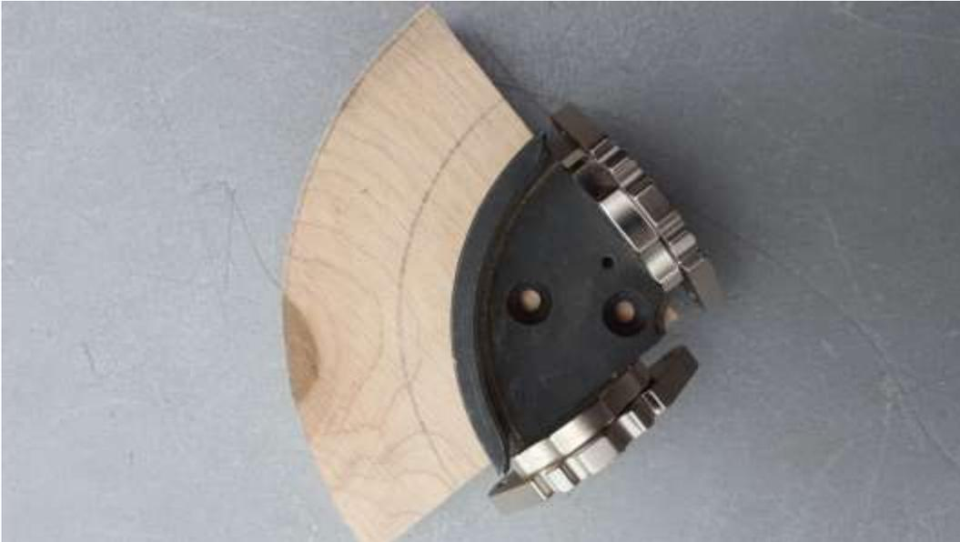
Use the drill press for better drilling, drill holes corresponding to the holes in the jaw being used. For Stronghold & Talon chucks. This is a number "C" Drill bit which is the correct size for 6 MM screws. Other chucks may use a different size screw. See the picture below.
