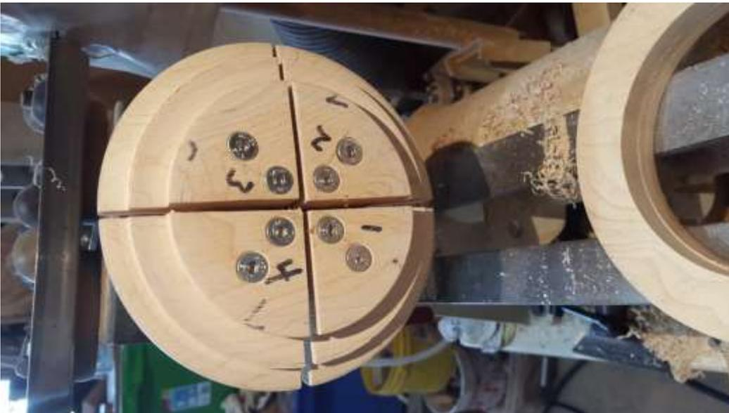
Place the top onto the step jaws.
