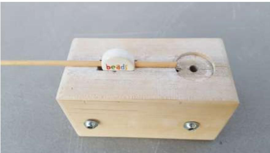
Below is a go-no-go gauge to insure that the beads will fit into the top of the knob. Note the 3/16inch hole through the wood to remove a stuck bead.
