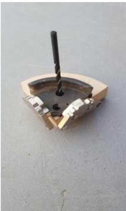
Counter sink all of the holes for the screws so that the screws will sit flush or below the surface of the wood being used.
