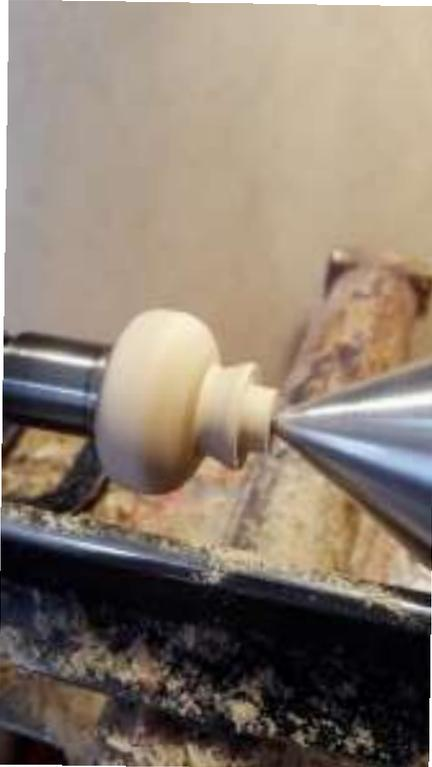
Use a Step type center drive and form the 1/2" inch or 9/16 inch tennon at the tailstock end. Sand the knob as needed for a good smooth finish.
