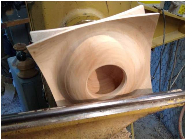
After an initial "V" cut with my  $\frac{1}{2}$ " Thompson bowl gouge with a 40/40 grind I did the rest of the hollowing with Mike Hunter's straight and swan neck "Baxter" carbide tools.
