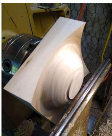
With the blank securely screwed onto the screw-chuck start turning the bottom of the wings and bowl including the tenon. The tenon will become the feet in the final step.
