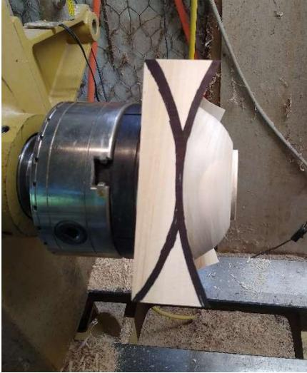
Using a Sharpie mark out the position of both bottom & top wings on one side of the blank. Make sure that they merge together at the center and that the top corners are slightly below the top (left in pic.) of the blank.
