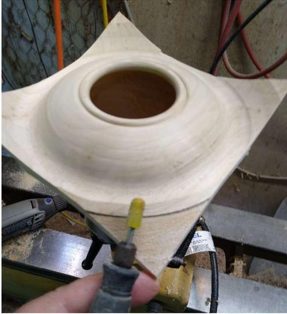
Using a rotary tool with a Saburrtooth cylindrical cutter you can quickly remove the excess leftover wing material. Finish the process with sandpaper.
