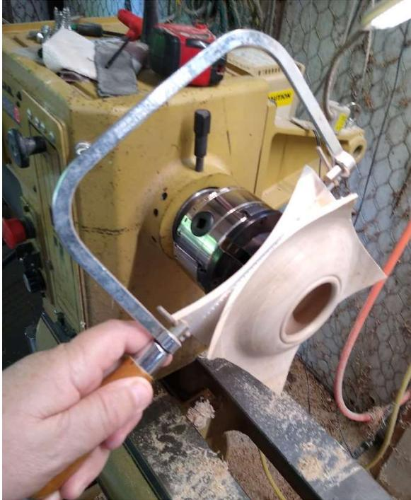
Removing the surplus wings! There's a number of ways to do this but I find a coping saw works great! I used the Indexing feature on my lathe for the first time ever to stop the piece from rotating while I sawed off the wings I didn't want.
