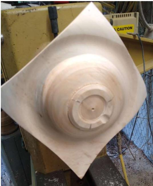
Almost there! Remount the piece in the lathe on an expanding chuck to clean up the tenon for carving into 3 feet.
